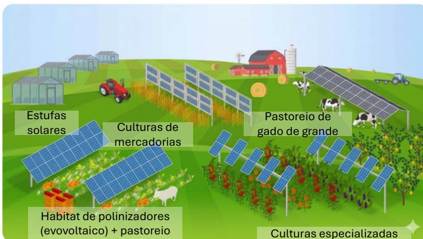
Figura 2: Esquema de agrivoltaico Adaptado de Illustration by Tom Hickey and Al Hicks, NREL , in Agrivoltaics Basics
